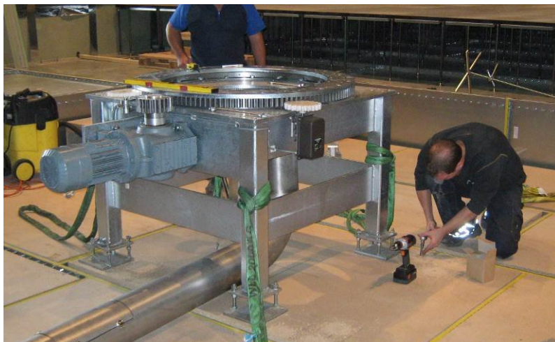
Fig.: Drive unit assembly of turntable
