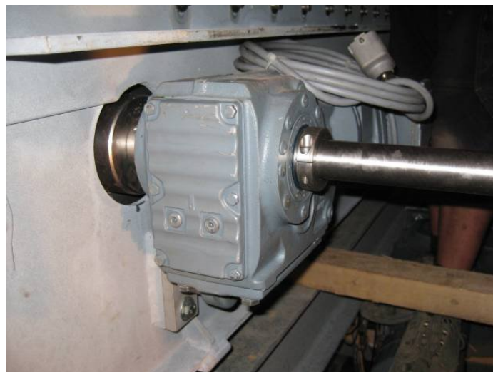
Fig.: Motor for wheelbase adjustment
