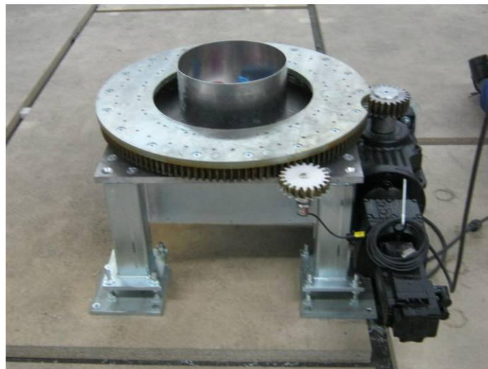
Fig.: Drive unit assembly of turntable
