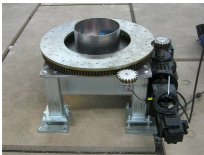
Fig.: Drive unit assembly of turntable
