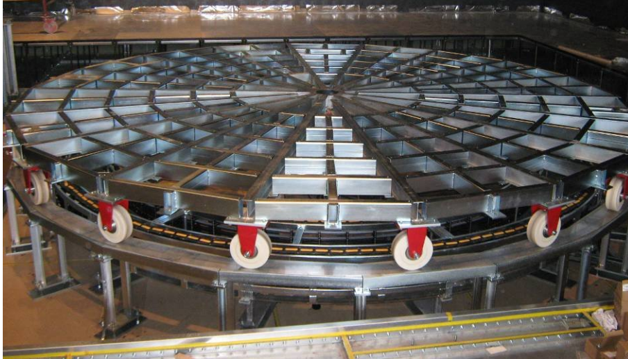
Figure: Turntable structure made of solid welded galvanised steel
