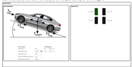
Additional to the coefficient setting method, a road angle and the force distribution at more wheel drives could be also set.
